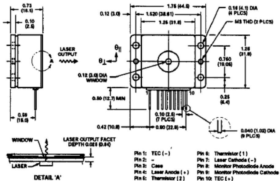
**The configuration and dimensions of a high-brightness diode laser (SDL 2400 series, 3.0 W continuous wave output optical power). Such power is considered for the cloud detection in EUSO.**
